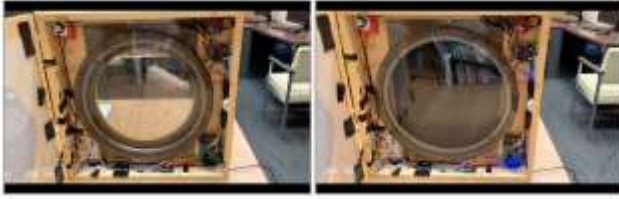
Fig. 2. Images showing the tinting effect in action. In the image on the left, the two polarizers are aligned along the same optical axis, maximizing light transmission. In the image on the right, one of the polarizers has been rotated to generate the tinting effect.
